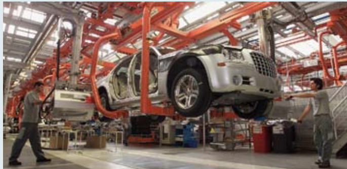
A Konecranes manipulator with a nutrunner for wheel assembly at Magna in Austria.
