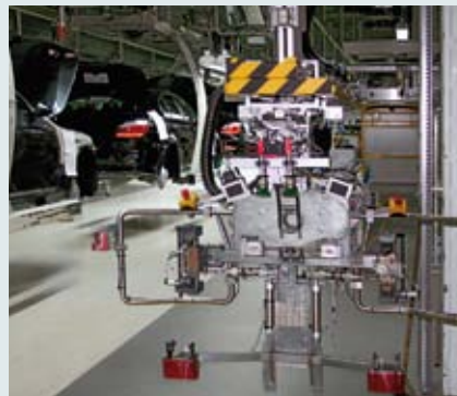
A Konecranes manipulator based on a Vertical Lifter for front-end module at BMW in Germany.
