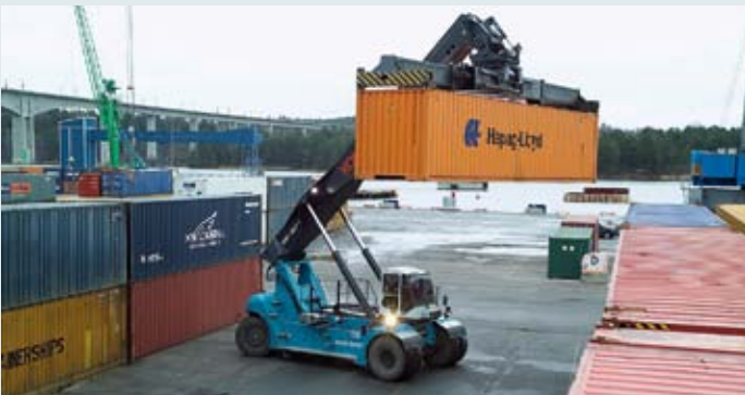
Konecranes reach stackers lift from 10 to 80 tons with top and bottom-lift. They can be fitted with special attachments for automotive processes.
