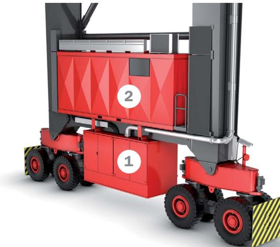
Figure 2. The diesel fuel saver is retrofitted in the genset enclosure (1) while the necessary modifications to the electrical systems are made in the e-house (2) above it. Some software modifications are also done at the same time.
