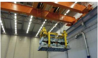
Cranes can also be equipped with a Die Gripper (or Die Lifter). The operator can control the width and length of gripper by a radio controller. Gripper legs are controlled by inverter. The needed positioning accuracy of a Die Gripper Crane is usually about +/- 20 mm realized with the following measures:
