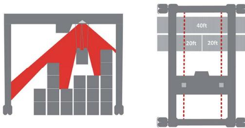
Figure 8. The Stack Profiling System remembers the layout of your container bay. Here is a sample layout from the side (left) and the top (right).
