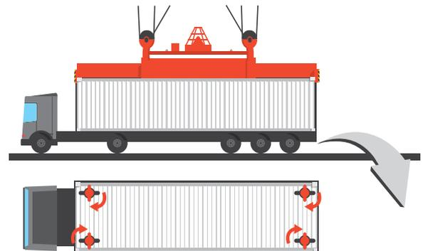
Figure 11. All twist locks must be disengaged before lifting. Trailer Lift Prevention stops lifting if a trailer lift is detected.
