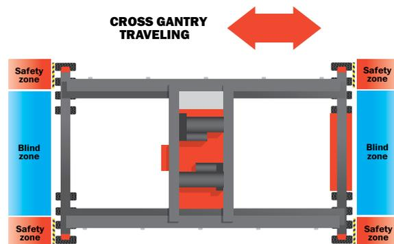
Figure 6 and 7. The safety zones are pre-programmed according to local regulations and your own yard requirements. Seen here: normal and cross gantry travel. "Rotate" is also available. In cross-gantry travel, the "blind zones" can be eliminated by adding more laser sensors.
