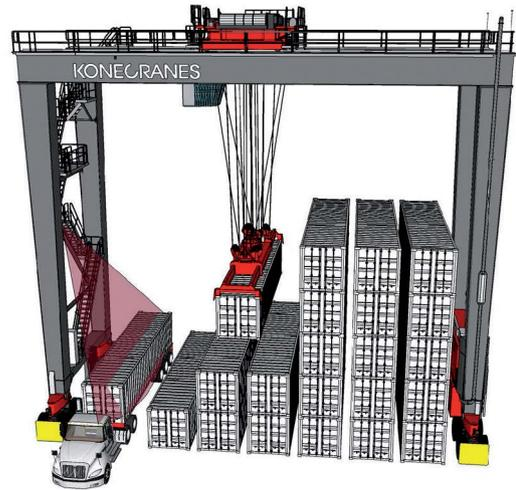
Figure 10. Auto Truck Guiding uses truck container scanning to tell the driver when to slow down.
