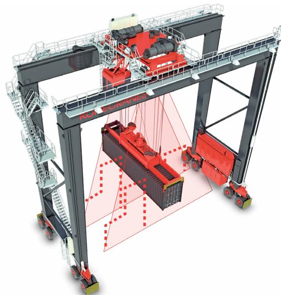
Figure 9. The Stack Collision Prevention system uses two laser scanners. They constantly monitor the containers in the stack when the trolley is in motion.
