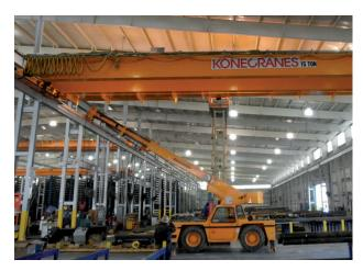
when Konecranes first inspected it, all four of its wheels were different sizes and the crane could not track properly. Breakdowns on EMJ's cranes were common.
